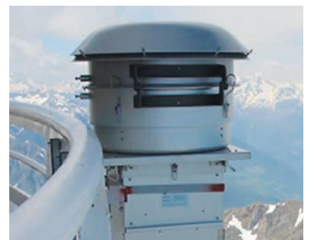
Intake for fine particle pump at Pic du Midi Observatory.
