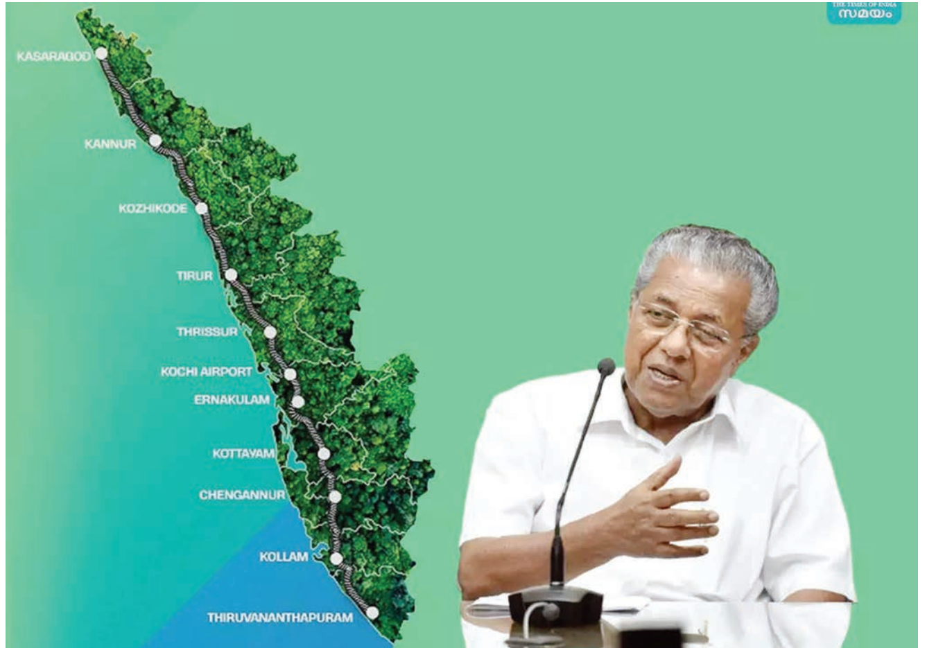
The 529.45 km SilverLine corridor connecting Kasaragod and Thiruvananthapuram, with an operating speed of 200kmph, eases the transport between North and South ends of the state and reduces the total travel time to less than 4 hours, compared with the present 10 to 12 hours. The intermediate stations include Kollam, Chengannur, Kottayam, Ernakulam, Kochi Airport, Thrissur, Tirur, Kozhikode and Kannur.
