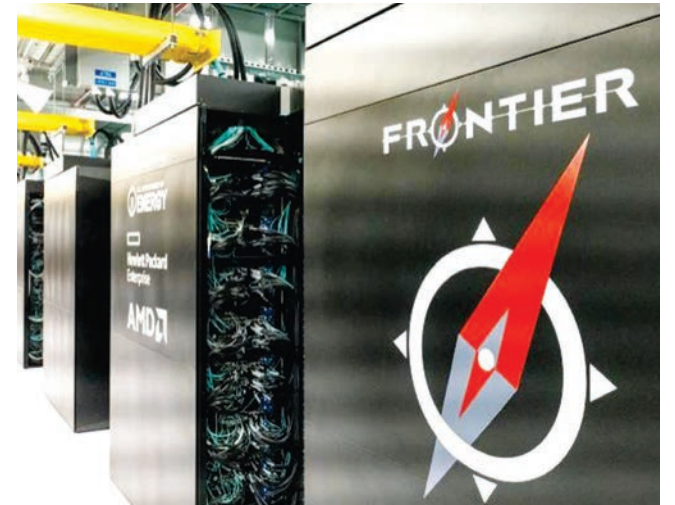
Frontier features a theoretical peak performance of 2 exaflops, or two quintillion calculations per second, making it 10 times more powerful than ORNL’s Summit system.
